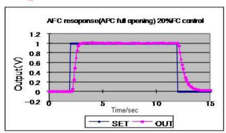
Flow Control devise: Actual flow rate result: 1000 SCCM FS
